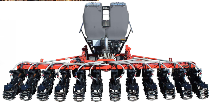
Gladiator® 1210 | 12-Row Strip Tillage System with 9-Ton Montag Gen II Fertilizer Tank
